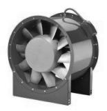
Medium pressure axial fan with axial impeller with 14 aerodynamically profiled blades from polymers. Dynamically balanced to DIN ISO 1940-1, class 6.3 for low-vibration operation. Totally enclosed 3-phase squirrel cage motor with built-in thermal contacts, maintenance-free, speed controllable by voltage reduction, with low-noise sealed for life ball bearings.
